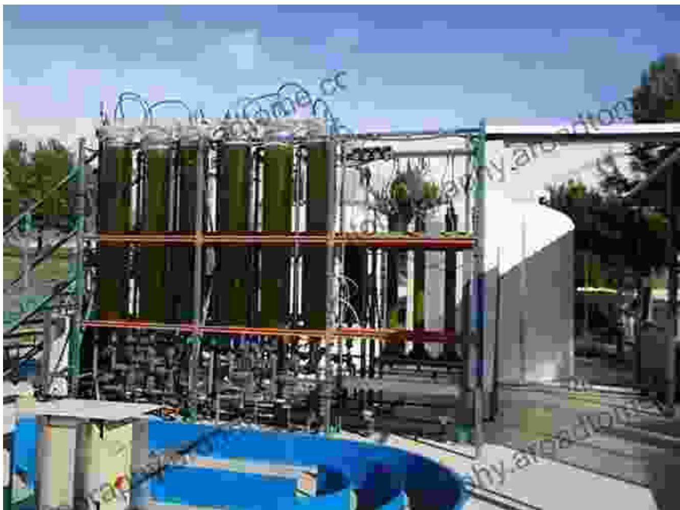
PBRs combine biofiltration with photosynthesis. Microalgae or cyanobacteria are grown in a bioreactor, which serves as the biofilter. The microorganisms utilize sunlight to photosynthesize, producing oxygen and consuming carbon dioxide. This process creates an ideal environment for microbial pollutant degradation, enhancing the biofilter's efficiency and sustainability.
